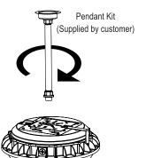
Feed fixture leads through customer supplied pendant kit, and thread until locked securely.
