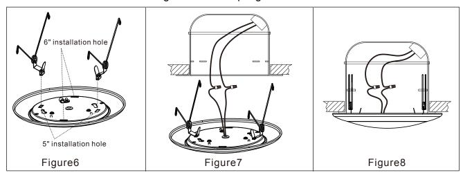
**WARNING:** Risk of fire or electric shock. Luminaire's wiring, ballast(s), or other electrical parts may be damaged when drilling for installation of reflector kit hardware. If drilling is required in any installation, check for enclosed wiring and components and be careful to protect them from any harm. To prevent wiring damage or abrasion, do not expose wiring to edges of sheet metal or other sharp objects.
