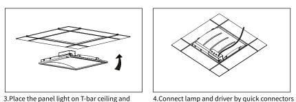
3.Place the panel light on T-bar ceiling and adjust its position
