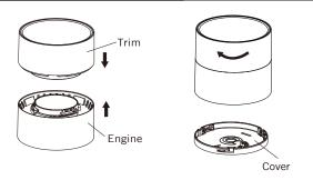
When trim and engine are separated, attached together, and secure them with clockwise direction.
