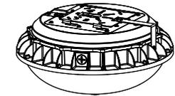
2. Feed fixture leads through customer supplied pendant kit, and thread until locked securely.
